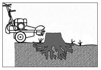
Place the machine into position with the cutting wheel near the top edge of the stump.
