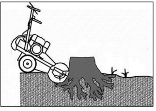
Conduct the pre-starting inspection if not already done and start the engine as per the operating instructions above. Allow the engine to "warm up" for 30 seconds with the engine revs set to the MIN position prior to starting to remove the stump.
