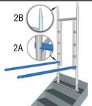
2. Position the frame with the foot assembly on the higher location on the staircase making sure that the frame head fitting always points toward the middle of the tower (2B). Fit 2 short horizontal braces to vertical tubes of the frame just above lowest rung ensuring spring loaded pin faces outward (2A).
