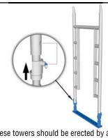
1. These towers should be erected by at least 2 competent persons. Fit an adjustable foot assembly into a walk through base frame ensuring that the spring loaded pins engage in the holes provided (1A).
