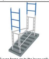
5. Fit a 3 rung frame on to the lower walk through base frame by locating onto head fitting with peg engaging into hold provided. Repeat the 6. Now fit a temporary platform, guardrail brace process at the other end using a 2 rung guardrail frame.
