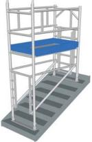
9. Fit the toeboards around the platform. Always remember to close the trapdoor immediately after climbing through.
