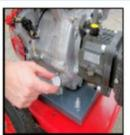
Check engine oil and replenish as required.
