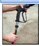
Attach trigger to high pressure hose.
