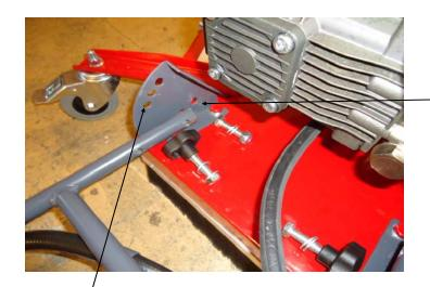
Place handle onto base and align holes with bracket.
