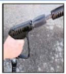
Release any pressure in hose by squeezing trigger and disconnect hoses from machine.
