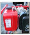
Check diesel using sight measure and replenish as required.
