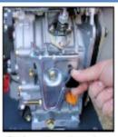
Push throttle into 'start' position and tighten knob.
