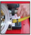
Place filter in bucket or water source & connect hose to machine & tighten
