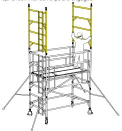
Fit 2 more AGR's to the end frames, with the top claws on the 10th rungs, lock the AGR's in place as in step 5. Fit a trapdoor deck on the 8th rung, with the trapdoor in line with the one below. Place a fixed deck on the 8th rung next to the trapdoor deck. The tower now has a platform height of 4.2m. If finishing at this height, move on to step 10. If greater platform height is required, repeat steps 7 and 8 until desired height is achieved.
